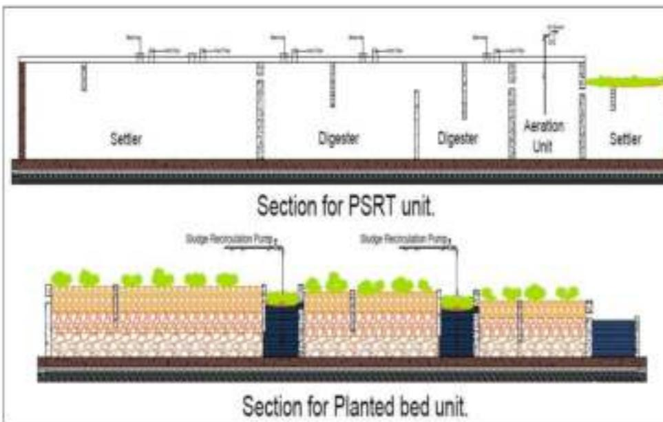
IWT are typical natural engineered treatment systems, designed and constructed to utilize the natural processes involving wetland vegetation, soils and their associated microbial assemblages to assist in treating the wastewater.
